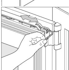
Now adjust the upper hinge so the sash either moves towards the upper hinge or away from it.
