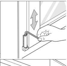
Next use an allen wrench to adjust the sash height.
