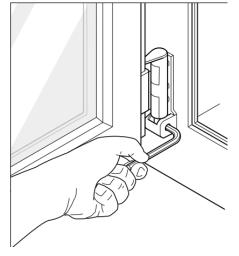
Use an allen wrench to adjust the sash towards the hinge or away from it.
