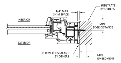
Then anchor the frame into the opening and apply some Dowsil 790 onto the head of the anchor screws and then affix the cap covers to the head of the screw.
